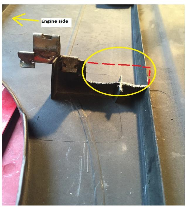
There is also a Styrofoam block that is sort of an "L" shape. This rests on top of the radiator (sorry, I didn't get a before pic – the yellow outline shows where the part of it was that I removed):
