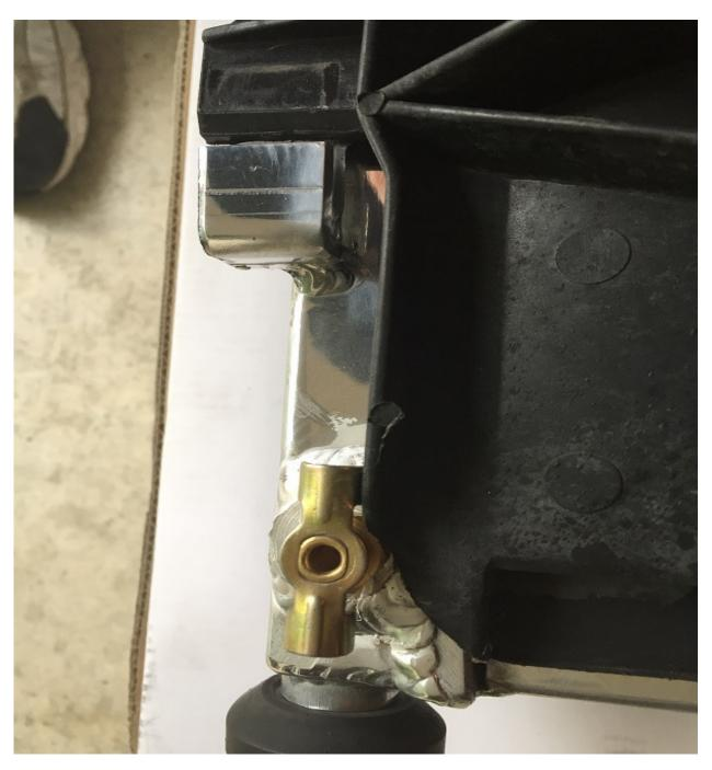
Simple solution – trim the shroud (marked in white). This is not a critical stress area so this should not create any issues:
