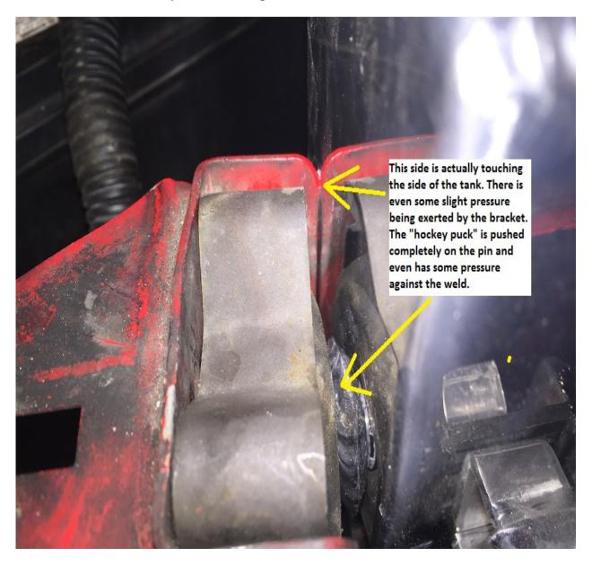
Solution – remove more sheet metal. I ground down about 3/16 of an inch from the bracket where it was touching the tank. This still left plenty of material for the bracket to maintain its integrity required to retain the "hockey puck" and spring clip. I now had about 1/16-1/8 of clearance between the bracket and the tank (I coated the ground edge with some black chassis paint):
