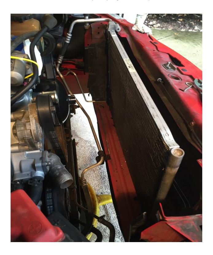
Test fit of the fan assembly before installation in the car – shroud is contacting the drain petcock preventing the assembly from dropping down enough for the tabs to engage the radiator retaining clips:
