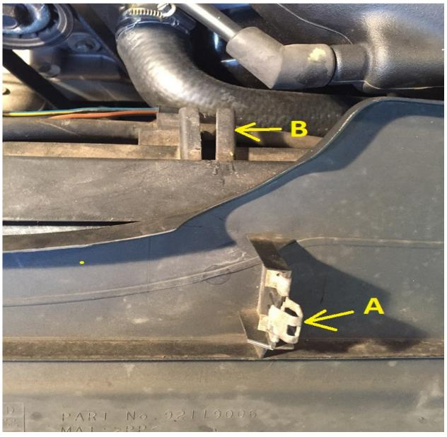
Since the fan shroud is now closer to the engine the clip attachment point is causing the top cover to be out of alignment.
