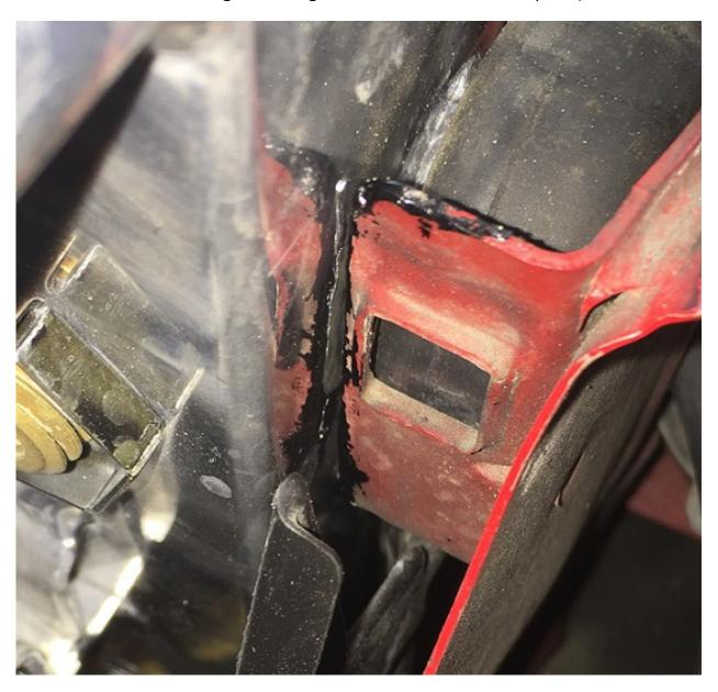
Due to the "hockey puck" being fully seated it is not possible for the radiator to shift toward the bracket and regain contact. The bottom mounting pins and bushings are fully seated, so now this seems to be a good fit with the radiator fully floating on all 4 rubber mounts.
