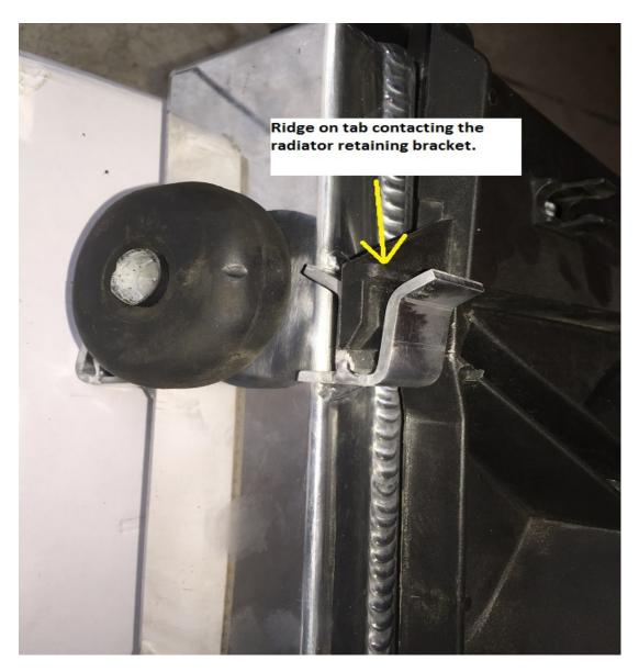
The factory radiator had brackets that allowed the tab to completely seat and then also locked it in by latching on to the ridge on the tab. I realize this type of bracket is not as easily duplicated in aluminum (factory is plastic), however after installation I can say that the fan assembly is sufficiently secured.
