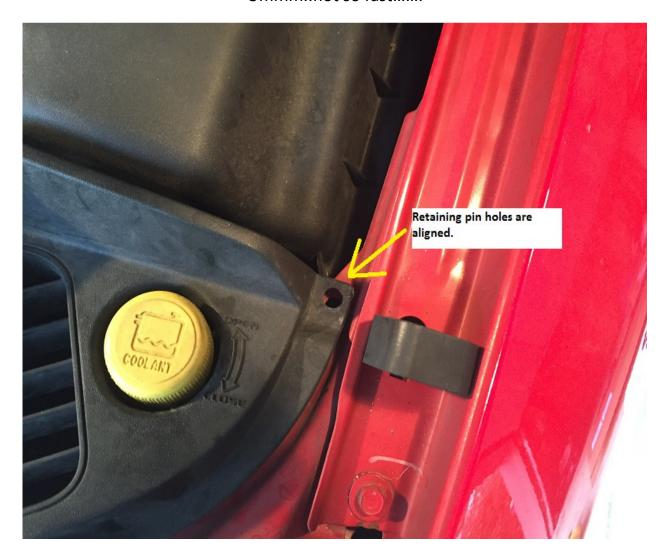
The driver side of the cover is located in place by the coolant recovery tank, and the retaining pin holes line up okay.
