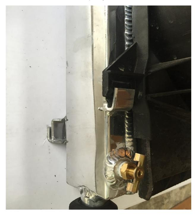
As you may have noticed from the previous picture, the tab does not slide all the way into the retaining bracket. This due to the location of the bracket. The top bracket stops the tab from fully engaging once the ridge on the tab contacts the bracket:
